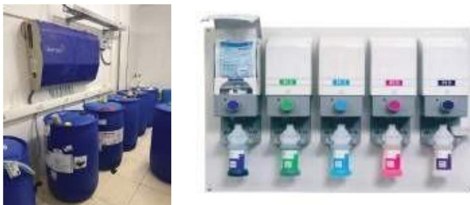
Figure 9. Laundry Dosing System and Bottle Usage
